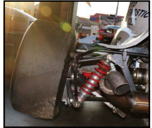
FM upright, halfshaft and CV joints are just some of the broken parts to be replaced. Photo by Brad Bernstein
