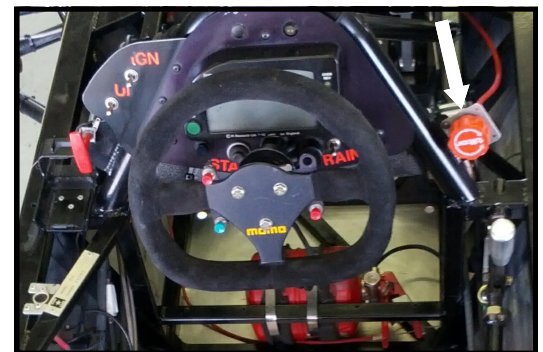
Arrow points to cockpit adjustable brake bias knob. Photo by Larry Mason
